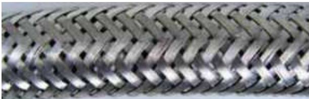
CF21.40.10.02.01.UL: after more than 10 million bending movements, no shield wire breakages
