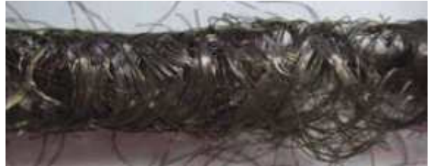
The detail inspection of the shield braid shows distinct damage on the shield wires.
