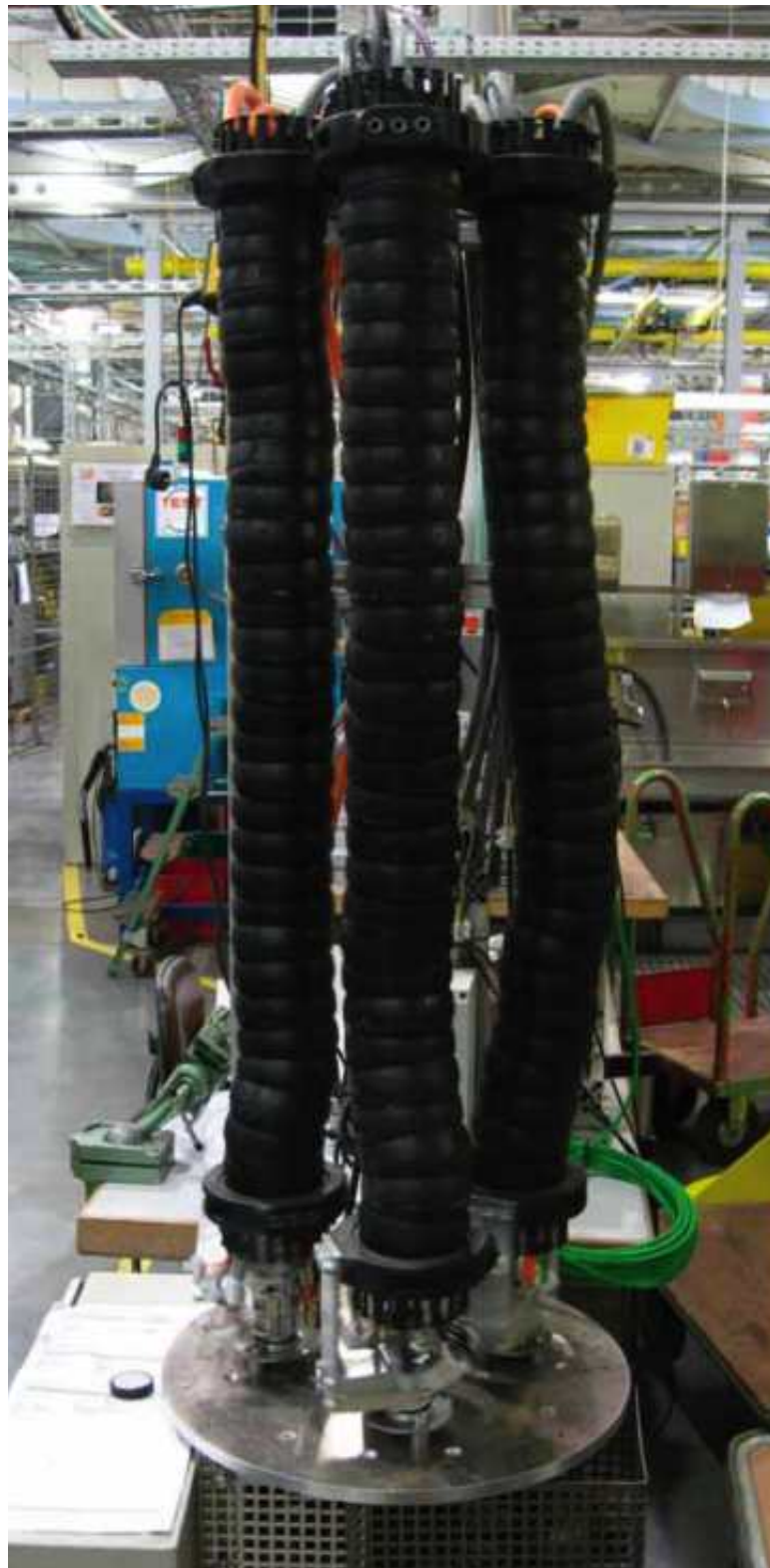
The "torsion test bench" especially developed according to the igus® standard.
