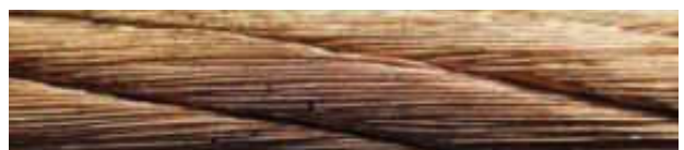
igus® test lab: The cables were tested in movements of \pm 270^\circ .
