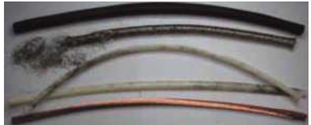
Picture 1: damaged overall shield sample of the braid version after 250,000 movements.
