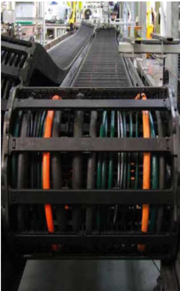
Deliberately non-conforming chain filling in order to simulate a real application.
