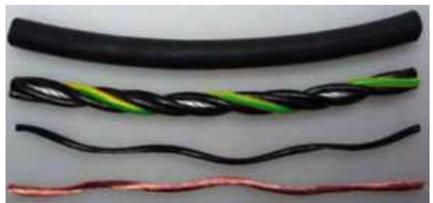
The individual elements of the CF9 from the cable piece dissected for the test setup.
