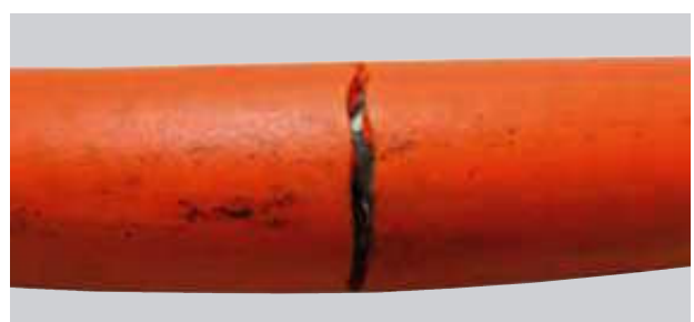
Cracks in the outer sheathing of materials from competitors caused by the "use of oil" in E-Chains®.
