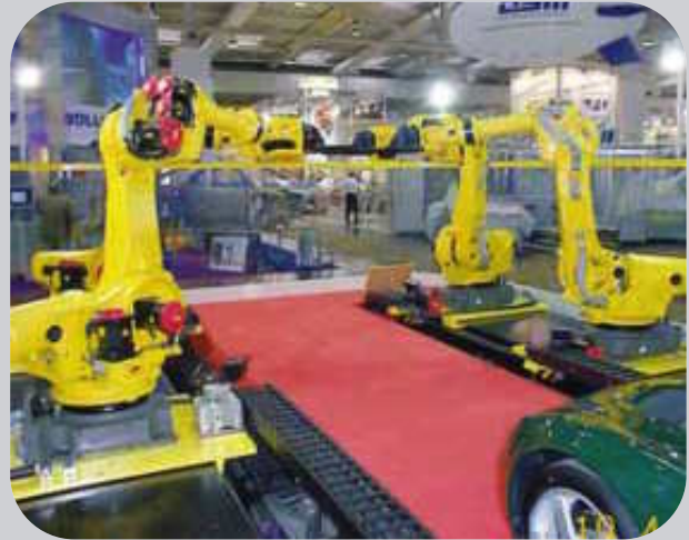
igus® ReadyChain® used for travel axles for 6-axes robots - standard filling with additional options
