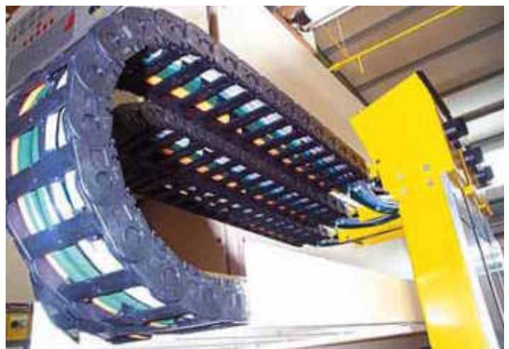
igus® Chainflex® cables also allow for minimum bending radii of 5 x d together with millions of strokes.
