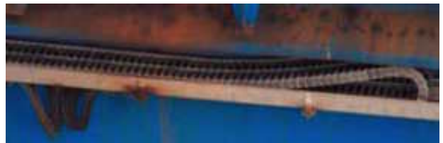
An igus® energy supply system with an approx. length of 26 m in a stainless steel trough with middle band support.
