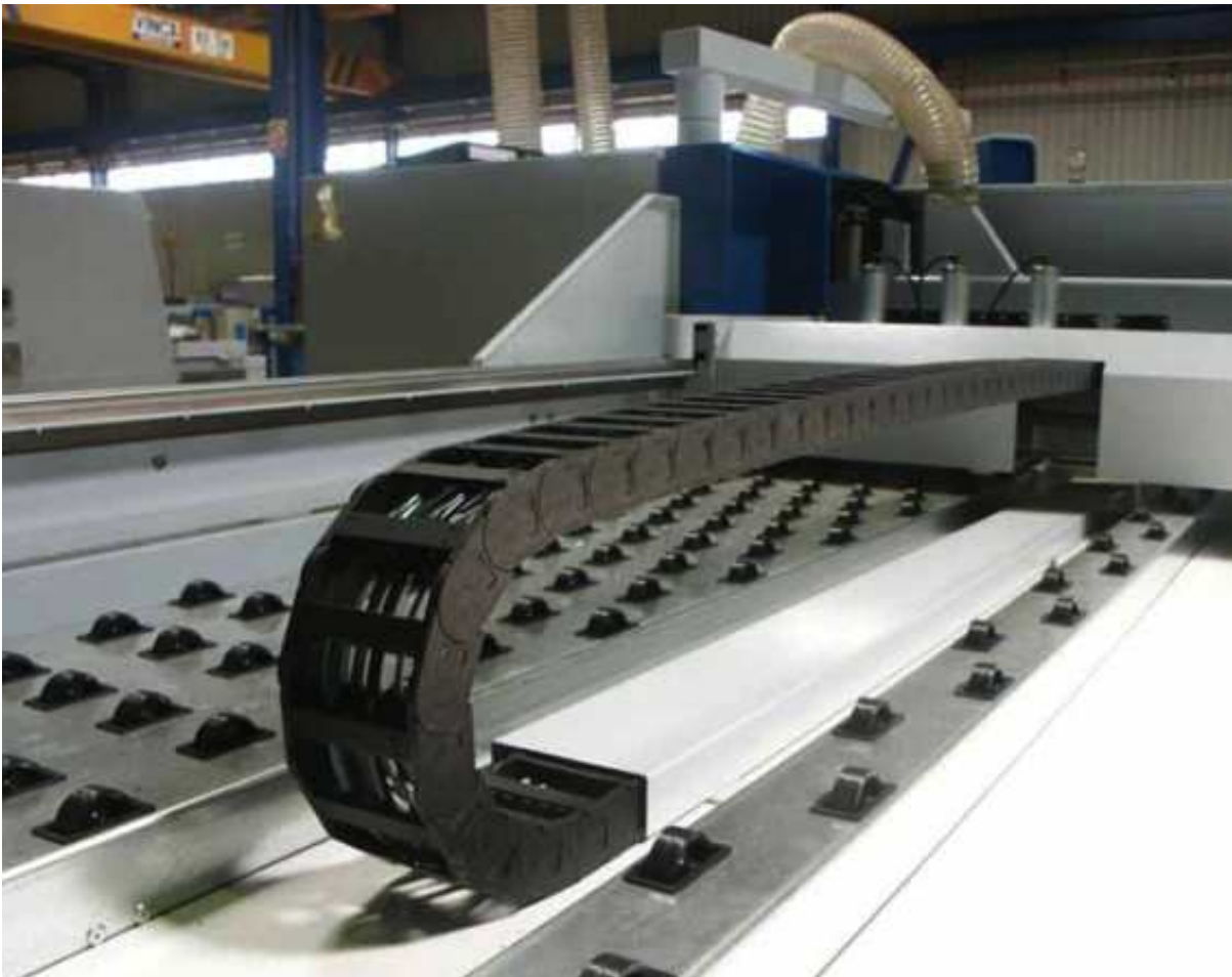
Chainflex® CF130.UL for woodworking. E-Chain®: E4/light
