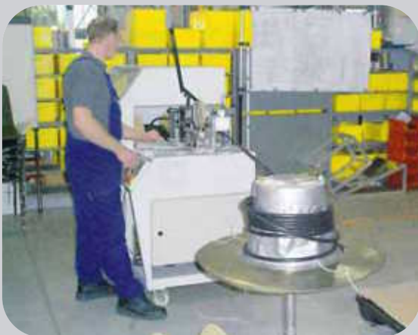
Non-spinning cable handling for more safety
