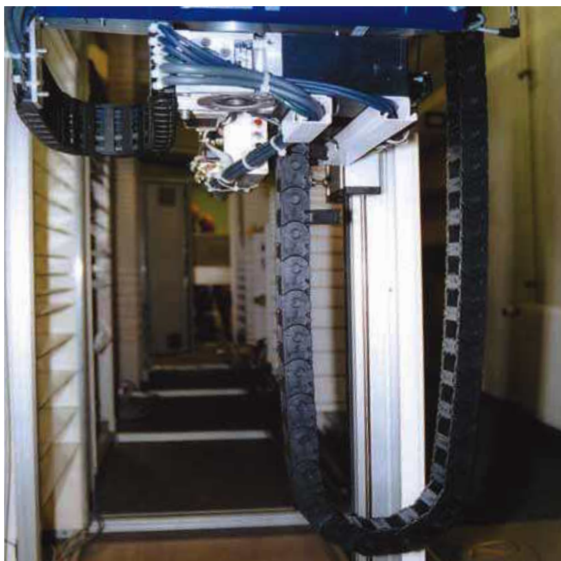
Metal-free fibre optic cables for fast handling applications. E-Chain®: System E2/000
