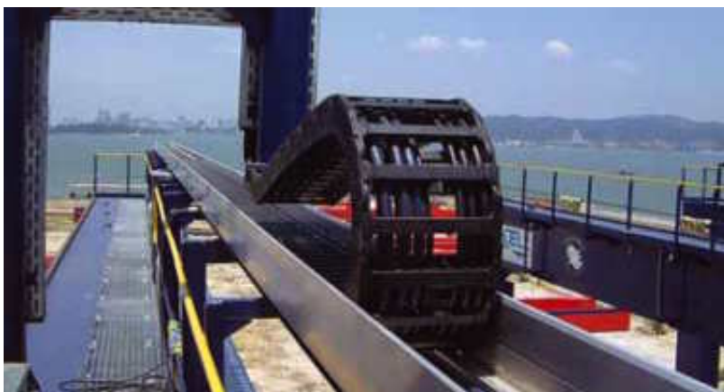
Chainflex® CF310.UL for outdoor crane systems. E-Chain®: Series E4/00
