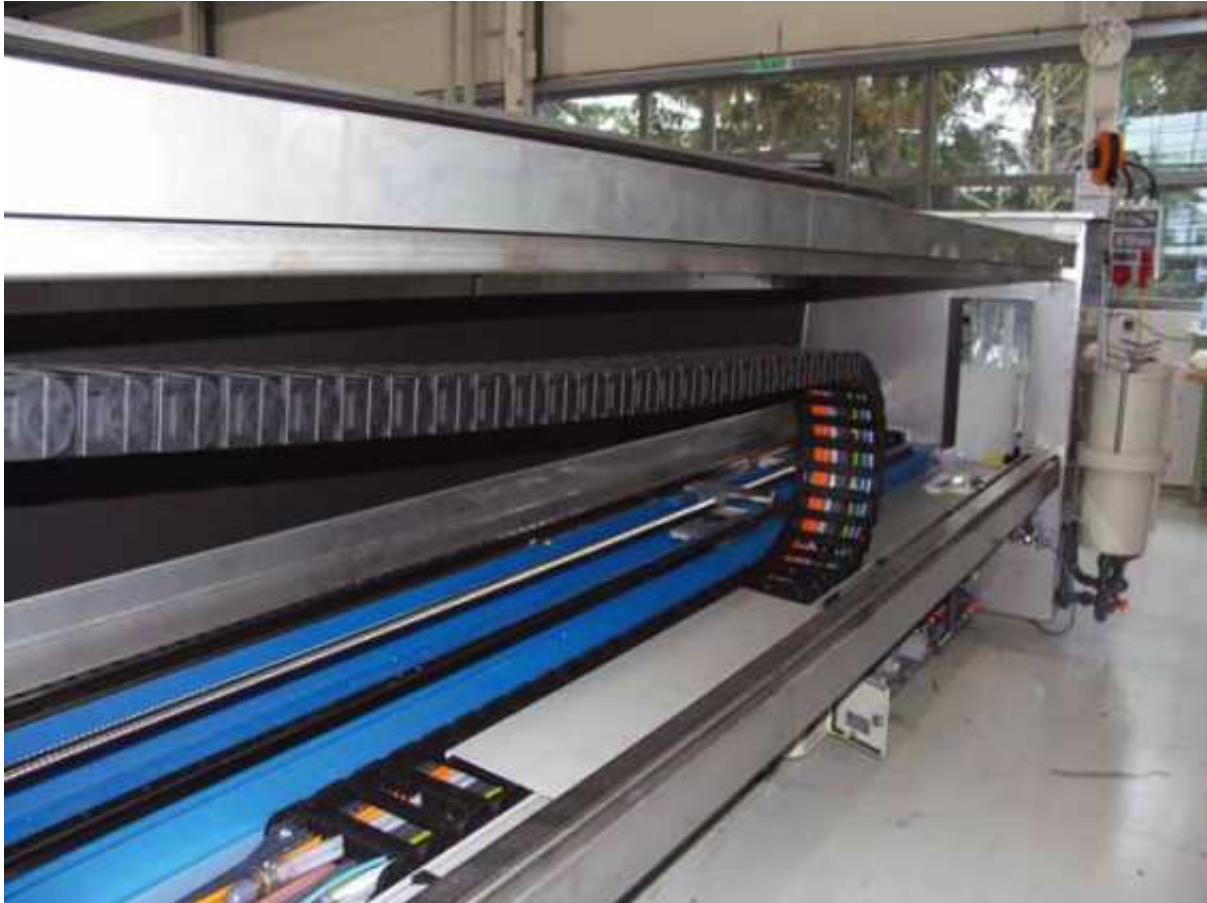
Pre-assembled energy chains with Chainflex® cables for special mechanical engineering applications.
