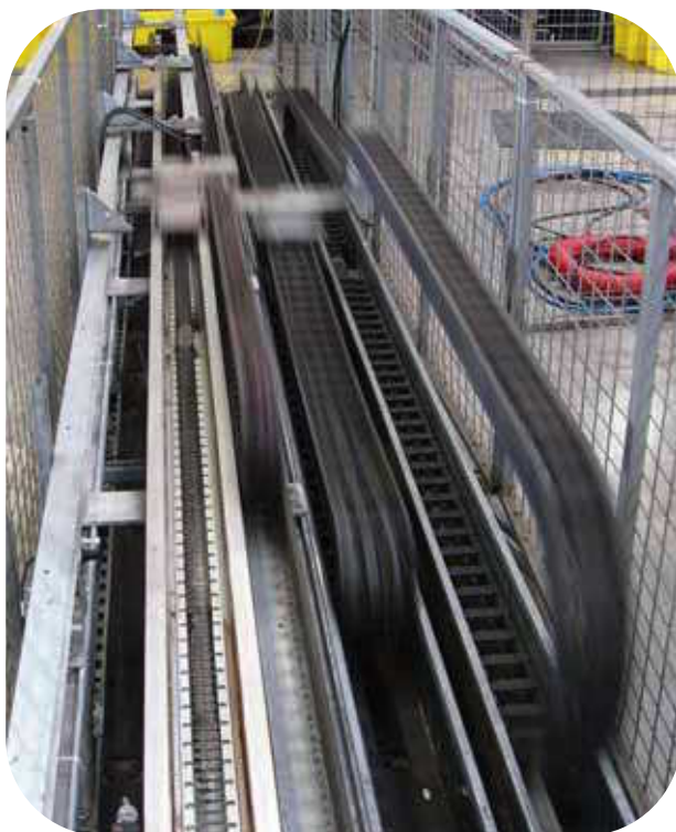
Picture: Sliding application as the basis of the test structure
