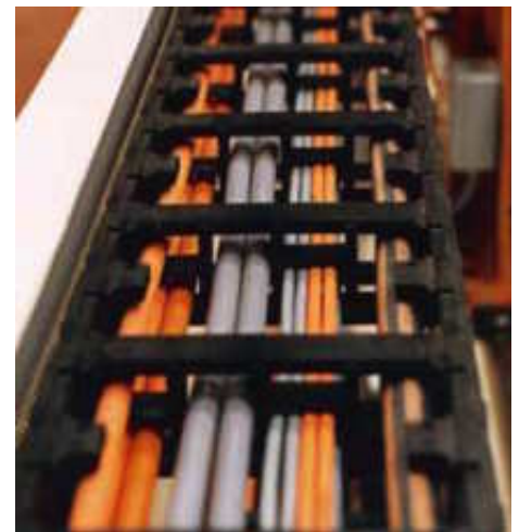
Perfectly installed cables with igus® interior separation
