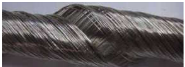
Picture 3: detail pictures of the CFROBOT after more than 3.0 million movements of \pm 270^\circ .
