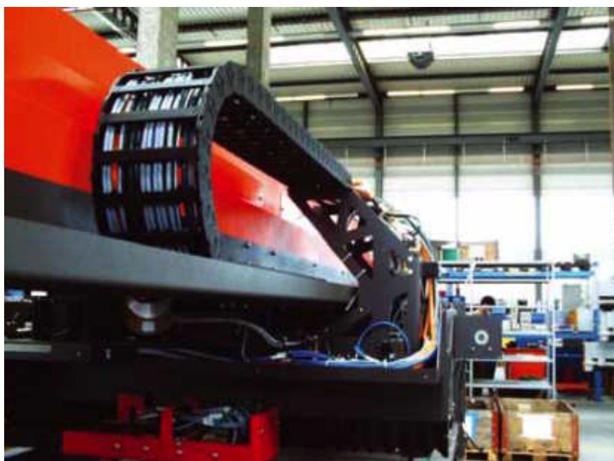
Chainflex® CFPE for machining units. E-Chain®: Series E2 medium
